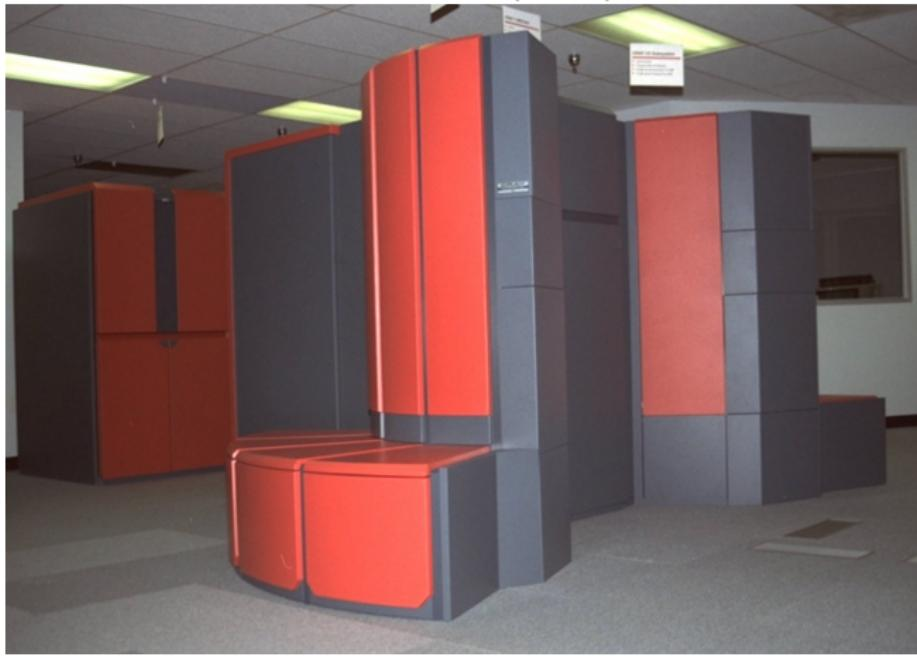
max. 8 vector processors, 2.6Gflop/s, 512MB RAM, 4GB SSD
