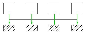
If each processor moves data from and to its own unique memory element, the **bandwidth multiplies**.
