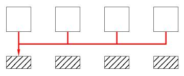
If each processor moves data to the same single memory element, the **bandwidth is limited** by that of a single memory controller.
