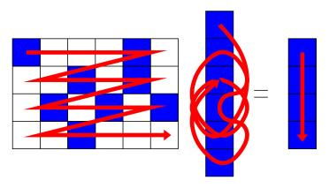
Accesses on the input vector are completely unpredictable.
