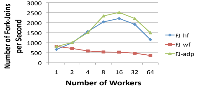
Fig. 7. Performance results for FJ(1024) microbenchmark (tasks are spawned iteratively) on Niagara 2 using 1 to 64 workers. Number of fork-joins performed per second is reported. (Bigger is better.)
